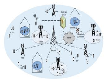
Fig. 2. Multi-tier cellular network architecture.
