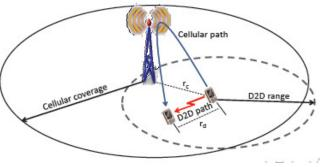
Fig. 3. Device-to-device (D2D) communication.
